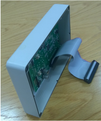
H10003SP Controller PCB low voltage board + Cover (pictures show back and front view)
