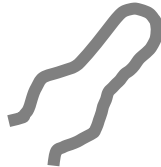
Ref 45 Clip for retaining the Diverter Actuator
