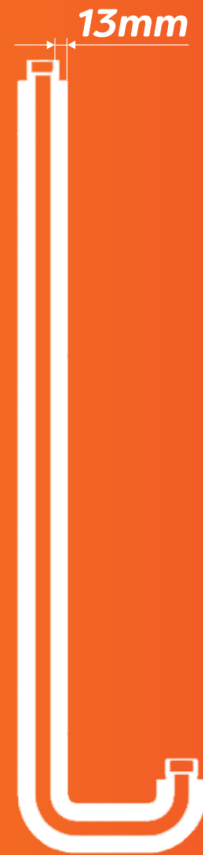
Top Entry Pipe with Insulation
